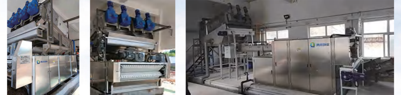
Project site of Spiral Sludge dehydrator
